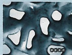
Video image of a reactive polymer flowing into an idealized porous medium. Courtesy of Karsten Thompson.
